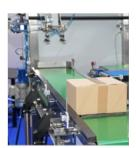
Combining 3D and active IR images can be used to create robust completeness checking systems. Check that each outbound packing container is fully loaded with the correct number of cartons or items before sealing and avoid costly customer returns.
